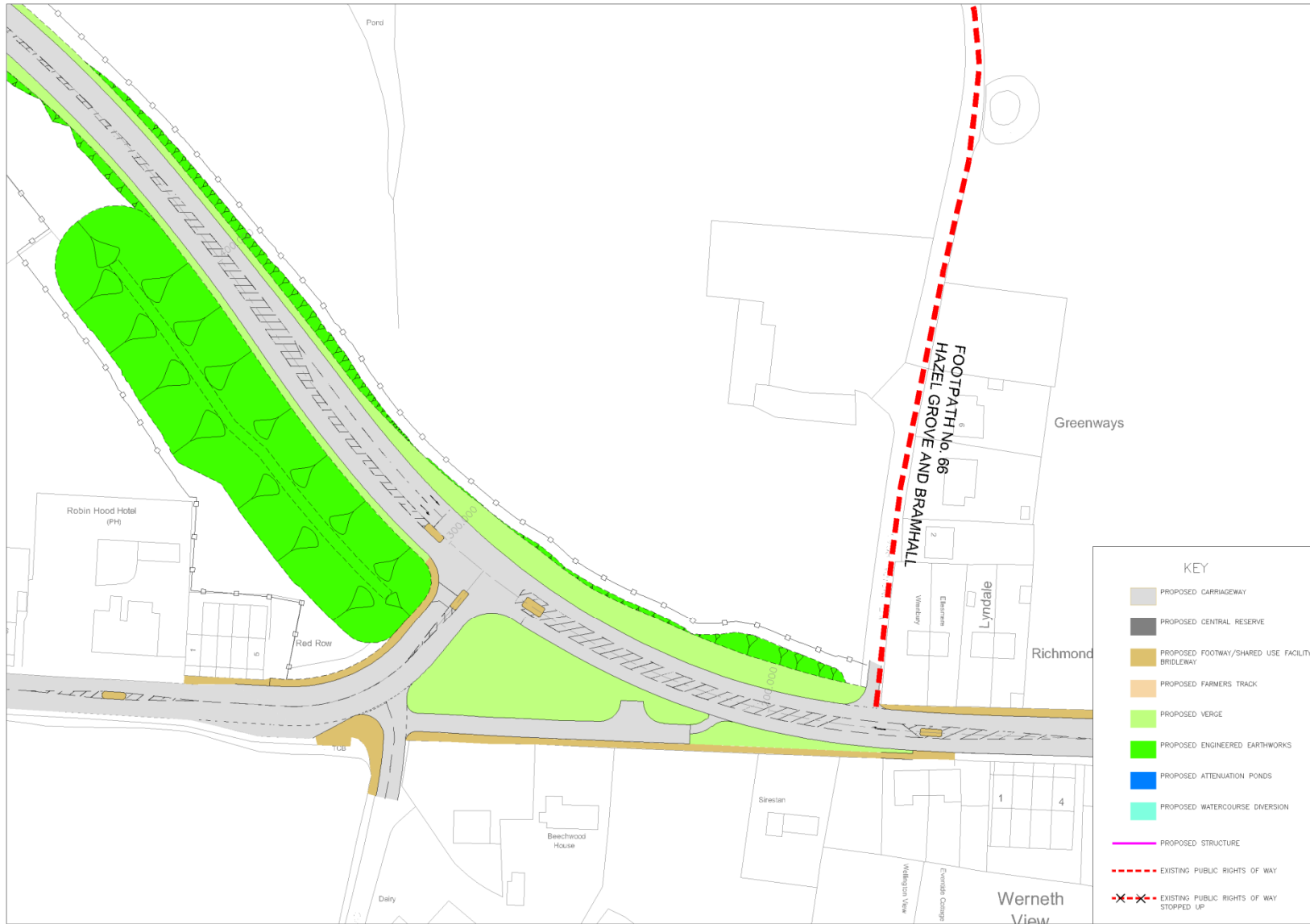
Figure 2.4 – Proposed Highway Route: Hazel Grove east (A6 Buxton Road) – Realigned A6/ Buxton Road (Eastern Tie-in Junction)
